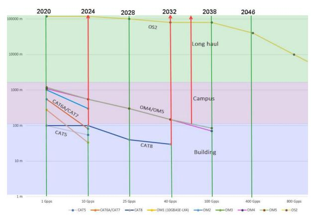
If we consider cable types in terms of future viability, the following picture emerges: The diagram shows possible cable lengths depending on cable type, with the year when certain bandwidth requirements are expected shown at the top.
